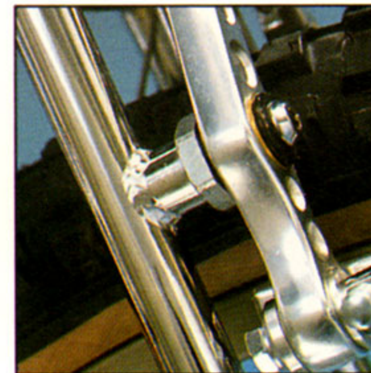
Heliarc welded cantilever mounts are more reliable than brazed-on mounts.
