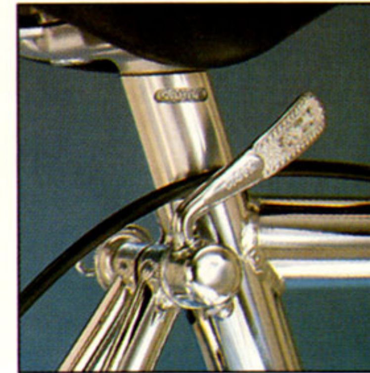
SR alloy seat pillar and Suntour quick release pin allows fast, tool-free seat adjustments.
